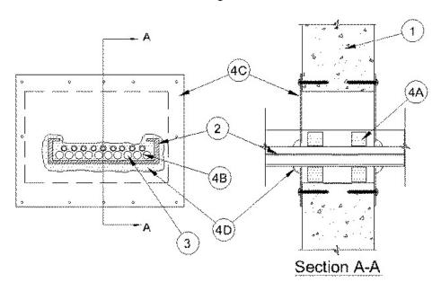
1. **Wall Assembly** — Min 4-1/2 in. thick reinforced lightweight or normal weight (100<u>150</u> pcf) concrete. Wall may also be constructed of any UL Classified Concrete Blocks\*. Max size of opening is 12 in. by 24 in.
