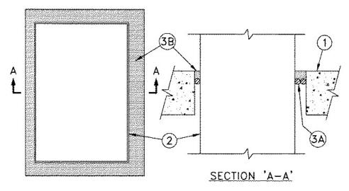
1. Floor or Wall Assembly — Min 4-1/2 in. thick reinforced light weight or normal weight (100<u>150</u> pcf) concrete. Floor may also be constructed of any min 8 in. thick UL Classified hollow core **Precast Concrete Units\***. Wall may also be constructed of any UL Classified **Concrete Blocks\***. Max area of opening is 384 sq. in. with max dimension of 32 in. When precast concrete units are used the max area of opening is 49 sq. in. with max dimension of 7 in.
