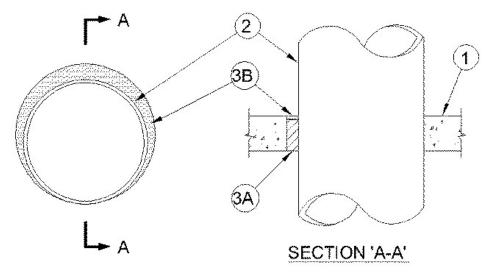
1. Floor or Wall Assembly — Min 4-1/2 in. (114 mm) thick floor or 5 in. (127 mm) thick wall of reinforced lightweight or normal weight (100-<u>150</u> pcf or 1600-2400 kg/m<sup>3</sup>) concrete. Wall may also be constructed of any UL Classified**Concrete Blocks**\*. Max diam of opening is 28 in. (711 mm).
