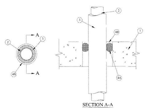
1. Floor or Wall Assembly — Min 4-1/2 in. thick reinforced lightweight or normal weight (100<u>150</u> pcf) concrete. Wall may also be constructed of any UL Classified **Concrete Blocks**\*. Max diam of opening is 6 in.
