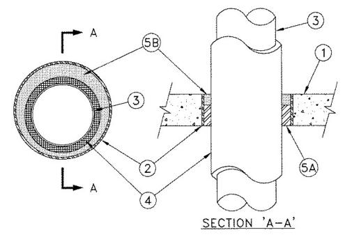
1. **Floor or Wall Assembly** — Min 2-1/2 in. (64 mm) thick reinforced lightweight or normal weight (100<u>150</u> pcf or 1600-2400 kg/m<sup>3</sup>) concrete floor or min 3-1/2 in. (89 mm) thick reinforced lightweight or normal weight concrete wall. Wall may also be constructed of any UL Classified **Concrete Blocks**\*. Max diam of opening is 8-1/4 in. (210 mm).
