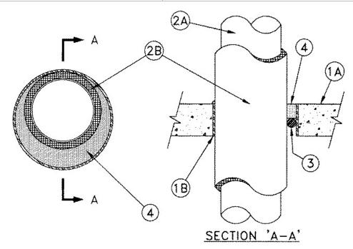
1. Floor or Wall Assembly — Min 4-1/2 in. thick reinforced lightweight or normal weight (100<u>150</u> pcf) concrete. Wall may also be constructed of any UL classified **Concrete Blocks\***. Max diam of opening is 17-1/2 in.
