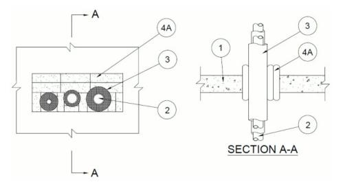
1. **Floor or Wall Assembly** — Min 4-1/2 in. (114 mm) thick reinforced lightweight or normal weight (100<u>150</u> pcf or 1600-2400 kg/m<sup>3</sup>) concrete floor or wall. Wall may also be constructed of any UL Classified**Concrete Blocks\*.** Max size of opening is 144 in<sup>2</sup> (929 cm<sup>2</sup>) with a max dimension of 18 in. (457 mm).
