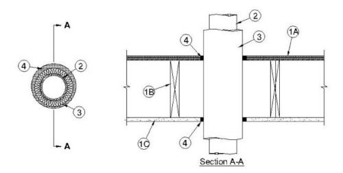
1. Floor-Ceiling Assembly — The 1 hr fire-rated wood joist floor-ceiling assembly shall be constructed of the materials and in the manner specified in the individual L500 Designs in the UL Fire Resistance Directory, as summarized below:
