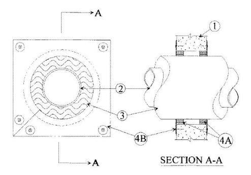
1. Wall Assembly — Min 7-5/8 in. thick wall assembly constructed of any UL Classified Concrete Blocks\*. Max diam of opening is 18 in.
