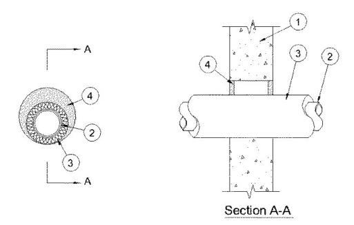
1. **Wall Assembly** — Min 4-1/2 in. (114 mm) thick reinforced lightweight or normal weight (100-<u>150</u> pcf or 1600-2400 kg/m<sup>3</sup>) concrete. Wall may also be constructed of any UL Classified **Concrete Blocks**\*. Max diam of opening is 8 in. (203 mm).
