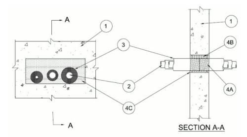
1. **Wall Assembly** — Min 6 in. (152 mm) thick lightweight or normal weight (100<u>150</u> pcf or 1600-2400 kg/m³) concrete. Wall may also be constructed of any UL Classified **Concrete Blocks\***. Max size of opening is 144 in² with a max dimension of 18 in. (457 mm).
