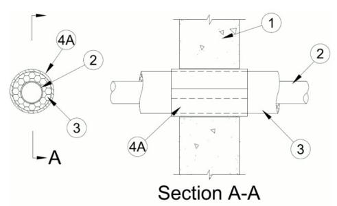
1. **Wall Assembly** — Min 6 in. (152 mm) thick lightweight or normal weight (100<u>150</u> pcf or 1600-2400 kg/m<sup>3</sup>) concrete. Wall may also be constructed of any UL Classified **Concrete Blocks\***. Diameter of the opening shall be 1/2 in. (13 mm) larger than OD of insulated penetrant. Max diam of opening is 6-1/2 in. (165 mm).
