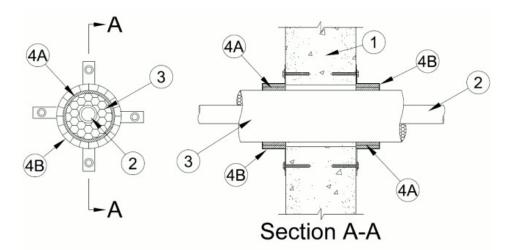
1. **Wall Assembly** — Min 6 in. (152 mm) thick lightweight or normal weight (100<u>150</u> pcf or 1600-2400 kg/m³) concrete. Wall may also be constructed of any UL Classified **Concrete Blocks\***. Diameter of the opening shall be max 1/2 in. (13 mm) larger than outer diameter (OD) of insulated penetrant. Max diam of opening is 4-1/2 in. (165 mm).
