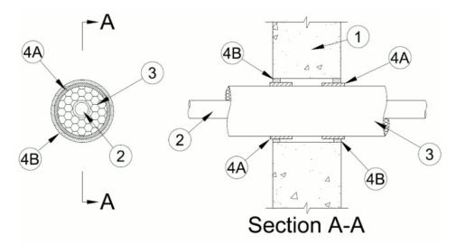
1. **Wall Assembly** — Min 6 in. (152 mm) thick lightweight or normal weight (100<u>150</u> pcf or 1600-2400 kg/m³) concrete. Wall may also be constructed of any UL Classified **Concrete Blocks\*.** Diameter of the opening shall be max 1/2 in. (13 mm) larger than outer diameter (OD) of insulated penetrant. Max diam of opening is 4-1/2 in. (165 mm).
