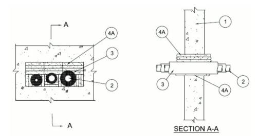
1. **Wall Assembly** — Min 6 in. (152 mm) thick lightweight or normal weight (100<u>150</u> pcf or 1600-2400 kg/m³) concrete. Wall may also be constructed of any UL Classified **Concrete Blocks**\*. Max size of opening is 144 irf with a max dimension of 18 in. (457 mm).
