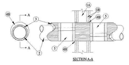
1. **Wall Assembly** — The 1 or 2 hr fire-rated gypsum board/stud wall assembly shall be constructed of the materials and in the manner described in the individual U300, U400 or V400 Series Wall and Partition Design in the UL Fire Resistance Directory and shall include the following construction features:
