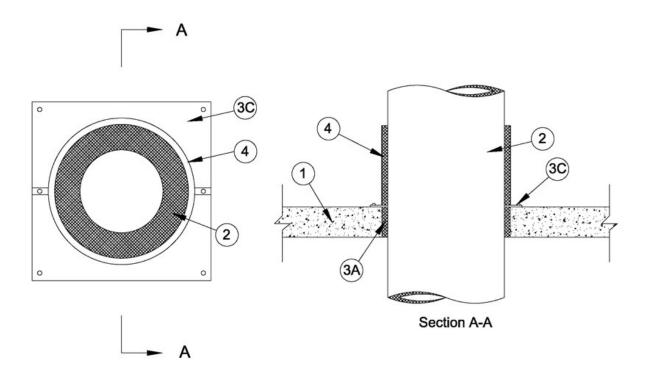
1. Floor or Wall Assembly — Min 4-1/2 in. (114 mm) thick reinforced lightweight or normal weight (100<u>150</u> pcf or 1600-2400 kg/m<sup>3</sup>) concrete. Wall may also be constructed of any UL Classified **Concrete Blocks**\*. Max area of opening is 13.75 ft<sup>2</sup> (1.28 m<sup>2</sup>) with max dimensions of 44-1/2 in. (1.13 m).
