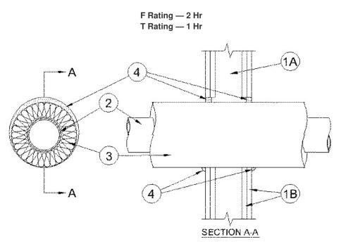
1. **Wall Assembly** — The 2 hr fire-rated gypsum board/stud wall assembly shall be constructed of the materials and in the manner specified in the individual U400 Series Wall and Partition Designs in the UL Fire Resistance Directory and shall include the following construction features:
