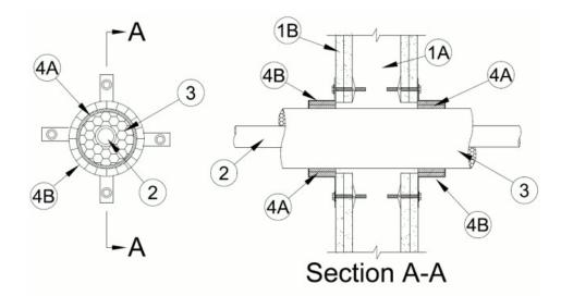
1. **Wall Assembly** — The 1 and 2 hr fire-rated gypsum board/stud wall assembly shall be constructed of the materials and in the manner specified in the individual U300, U400, V400 or W400 Series Wall and Partition Designs in the UL Fire Resistance Directory and shall include the following construction features:
