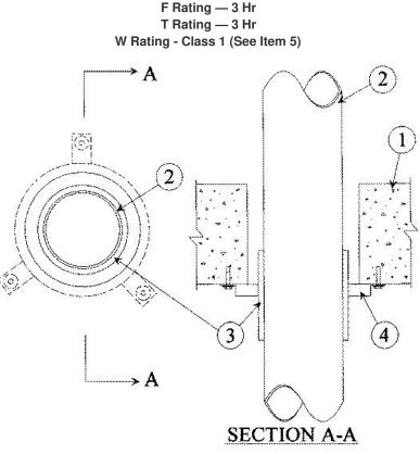
1. Floor or Wall Assembly — Min 4-1/2 in. (114 mm) thick reinforced lightweight or normal weight (100<u>150</u> pcf or 1600-2400 kg/m<sup>3</sup>) concrete. Wall may also be constructed of any UL Classified**Concrete Blocks**\*. Max diam of opening is 4-1/2 in. (114 mm).
