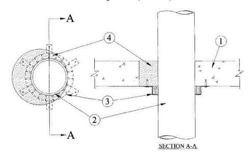
1. Floor or Wall Assembly — Min 4-1/2 in. thick reinforced lightweight or normal weight (100<u>150</u> pcf) concrete. Wall may also be constructed of any UL Classified **Concrete Blocks\*.** Max diam of opening is 10 in.
