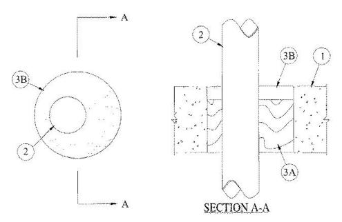
1. **Floor or Wall Assembly** — Min 4-1/2 in. thick reinforced lightweight or normal weight (100<u>-150</u> pcf) concrete floor or min 5 in. thick reinforced lightweight or normal weight (100-<u>150</u> pcf) concrete wall. Wall may also be constructed of any UL Classified **Concrete Blocks**\*. Max diam of opening is 4 in.
