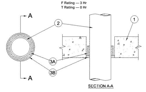
1. **Floor or Wall Assembly** — Min 4-1/2 in. thick reinforced lightweight or normal weight (100<u>-150</u> pcf) concrete floor or min 5 in. thick reinforced lightweight or normal weight (100-<u>150</u> pcf) concrete wall. Wall may also be constructed of any UL Classified **Concrete Blocks\***. Max diam of opening shall be 6 in.
