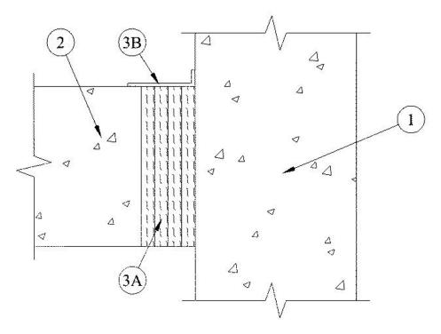
1. **Wall Assembly** — Min 6 in. (152 mm) thick reinforced lightweight or normal weight (100 <u>-150</u> pcf or 1600-2400 kg/m³) structural concrete. Wall may also be constructed of any UL Classified **Concrete Blocks**\*.
