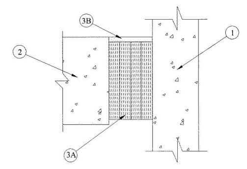
1. Wall Assembly — Min 6 in. thick reinforced lightweight or normal weight (100 -<u>150</u> pcf) structural concrete. Wall may also be constructed of any UL Classified Concrete Blocks\*.
