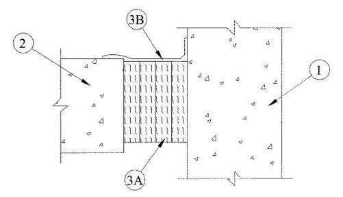
1. **Wall Assembly** — Min 4-1/2 in. (114 mm) thick reinforced lightweight or normal weight (100 <u>-150</u> pcf or 1600-2400 kg/m<sup>3</sup>) structural concrete. Wall may also be constructed of any UL Classified **Concrete Blocks**\*.
