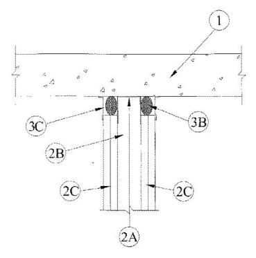
1. Floor Assembly — Min 5-1/2 in. thick reinforced light weight or normal weight (100<u>150</u> pcf) structural concrete.
