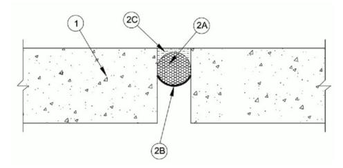
1. Floor Assembly — Min 6 in. (152 mm) thick reinforced lightweight or normal weight (100<u>150</u> pcf 1600-2400 kg/m<sup>3</sup>) structural concrete.
