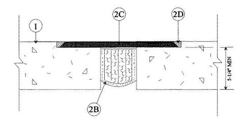
1. **Floor Assembly** — Reinforced lightweight or normal weight (100-<u>150</u> pcf) structural concrete having a min thickness of 5-1/4 in. at stepped-edges receiving Fill, Void or Cavity Material (Item 2C).
