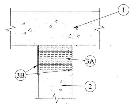
1. Floor Assembly — Min 4-1/2 in. (114 mm) thick reinforced lightweight or normal weight (100<u>150</u> pcf or 1600-2400 kg/m3) structural concrete. Floor may also be constructed of any min 6 in. (152 mm) thick UL Classified hollow-core **Precast Concrete Units\***.
