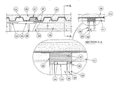
1. Floor Assembly — The fire-rated fluted steel deck/concrete floor assembly shall be constructed of the materials and in the manner described in the individual D700 Series Floor-Ceiling Design in the UL Fire Resistance Directory. The hourly fire rating of the floor assembly shall be equal to or greater than the hourly fire rating of the wall assembly. The floor assembly shall include the following construction features:
