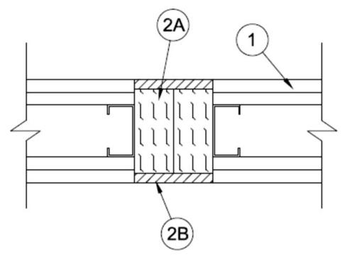
1. **Wall Assembly** — Nonbearing 1, 2 or 3 hr fire rated gypsum board/steel stud wall assembly constructed of the materials and in the manner described in the individual U400 or V400 Series Wall and Partition Designs in the UL Fire Resistance Directory and shall include the following construction features:
