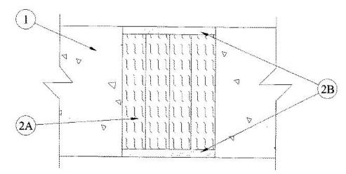
1. Wall Assembly — Min 4-1/2 in. thick reinforced lightweight or normal weight (100 -150 pcf) structural concrete. Wall may also be constructed of any UL Classified Concrete Blocks\*.
