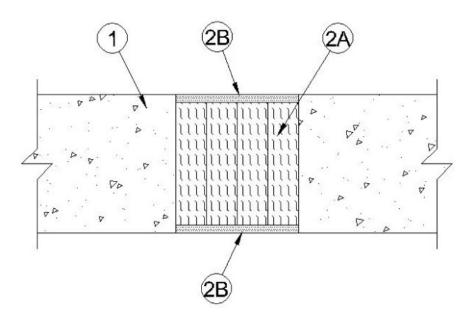
1. **Wall Assembly** — Min 4-1/2 in. (114 mm) thick steel-reinforced lightweight or normal weight (100<u>150</u> pcf or 1600-2400 kg/m<sup>3</sup>) structural concrete. Wall may also be constructed of any UL Classified **Concrete Blocks**\*.
