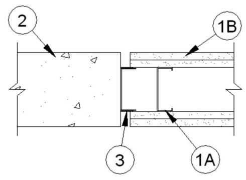
1. **Wall Assembly** — The 1 or 2 hr fire-rated gypsum board/steel stud wall assembly shall be constructed of the materials and in the manner described in the individual U400 or V400 Series Wall and Partition Design in the UL Fire Resistance Directory and shall include the following construction features:
