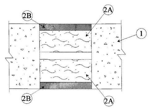
1. **Wall Assembly** — Min 4-1/2 in. thick lightweight or normal weight (100<u>150</u> pcf) concrete wall or min 7-5/8 in. thick masonry wall. Wall may also be constructed of any UL Classified **Concrete Blocks**\*. See **Concrete Blocks** (CAZT) category in the Fire Resistance Directory for names of manufacturers.
