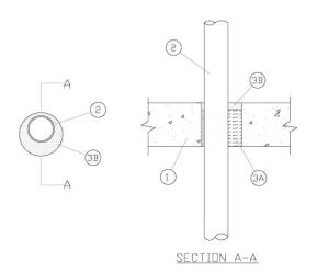
1. Floor or Wall Assembly — Min 4-1/2 in. (114 mm) thick floor, or min 5-1/8 in. (130 mm) thick wall, constructed of reinforced lightweight or normal weight (100-150 pcf or 1600-2400 kg/m3) concrete. Wall may also be constructed of any UL Classified Concrete Blocks\*. Max diam of opening is 4 in. (102 mm).
