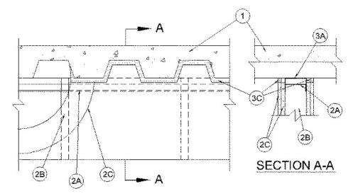
1. Floor Assembly — The fire-rated fluted steel deck/concrete floor assembly shall be constructed of the materials and in the manner described in the individual Floor-Ceiling Design in the UL Fire Resistance Directory and shall include the following construction features: A. Steel Floor And Floor Units\* — Max 3 in. (76 mm) deep galv steel fluted floor units.
