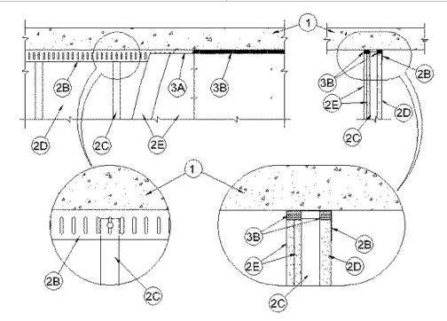
1. Floor Assembly — Min 4-1/2 in. (114 mm) thick reinforced lightweight or normal weight (100<u>150</u> pcf or 1600-2400 kg/m<sup>3</sup>) structural concrete.
