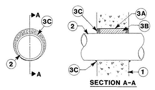
1. Wall Assembly — Min 5 in. thick reinforced lightweight or normal weight (100<u>150</u> pcf) concrete. Wall may also be constructed of any UL Classified **Concrete Blocks\*.** Max diam of opening is 20 in.
