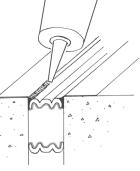
IMPORTANT: Sealant left between the wrinkles of the bellows could constrain movement — using a caulk knife, remove excess sealant and blend what remains into the bellows.
