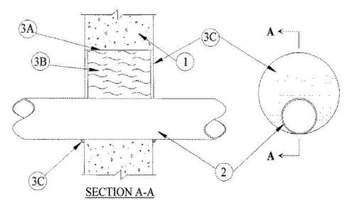
1. **Wall Assembly** — Min 5 in. thick reinforced lightweight or normal weight (100<u>-150</u> pcf) concrete. Wall may also be constructed of any UL Classified Concrete Blocks\*. Diam of circular through opening to be min 3/8 in. to max 2-3/4 in. larger than diam of through penetrants (Item 2).
