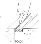
**NOTE** – Sealant band is only applied to the weather side of the DFR foam. No sealant band is needed on the other side.
