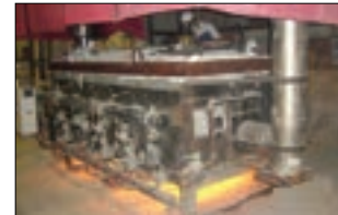
Testing oven below the Emshield DFR reaches a maximum temperature of 1850°F (1010°C).
