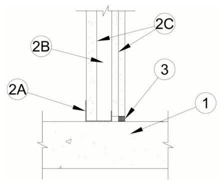
1. **Floor Assembly** — Min 4-1/2 in. (114 mm) thick reinforced lightweight or normal weight (100<u>150</u> pcf or 1600-2400 kg/m³) structural concrete. Floor may also be constructed of any min 6 in. (152 mm) thick UL Classified hollow-core **Precast Concrete Units**\*.
