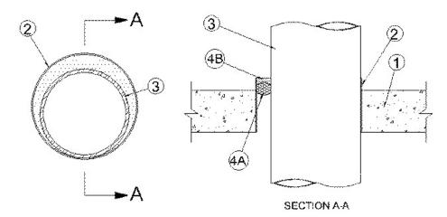
1. **Floor or Wall Assembly** — Min 4-1/2 in. (114 mm) thick reinforced lightweight or normal weight (100<u>150</u> pcf or 1600-2400kg/m³) concrete. Wall may also be constructed of any UL Classified **Concrete Blocks**\*. Floor may also be constructed of any min 6 in. (152 mm) thick UL Classified hollow-core **Precast Concrete Units**\*.
