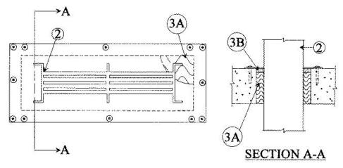
1. **Floor or Wall Assembly** — Min 4-1/2 in. (114 mm) thick reinforced lightweight or normal weight (100<u>150</u> pcf or 1600-2400 kg/m<sup>3</sup>) concrete floor or min 5 in. (127 mm) thick reinforced lightweight or normal weight concrete wall. Wall may also be constructed of any UL Classified **Concrete Blocks**\*. Max area of opening is 360 sq in. (2323 cm<sup>3</sup>) with max dimensions of 30 in. (762 mm)
