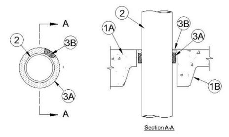
System tested with a pressure differential of 2.5 Pa between the exposed and the unexposed surfaces with the higher pressure on the exposed side.
