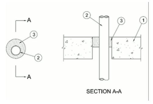
System tested with a pressure differential of 50 Pa between the exposed and the unexposed surfaces with the higher pressure on the exposed side.
